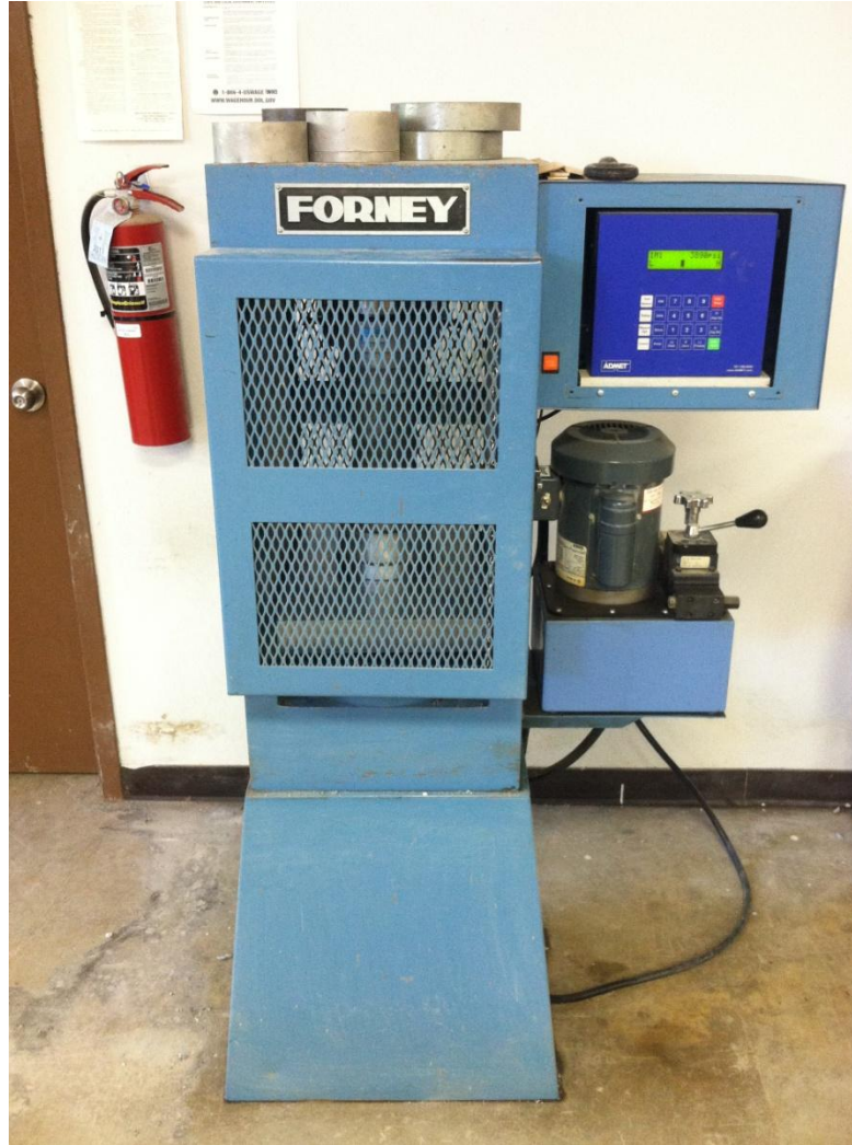
Figure 3.5 Concrete Testing Machine
