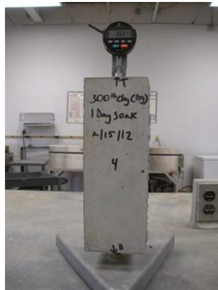
Figure 2.7 Linear Comparator and Prism used in ASTM C157
