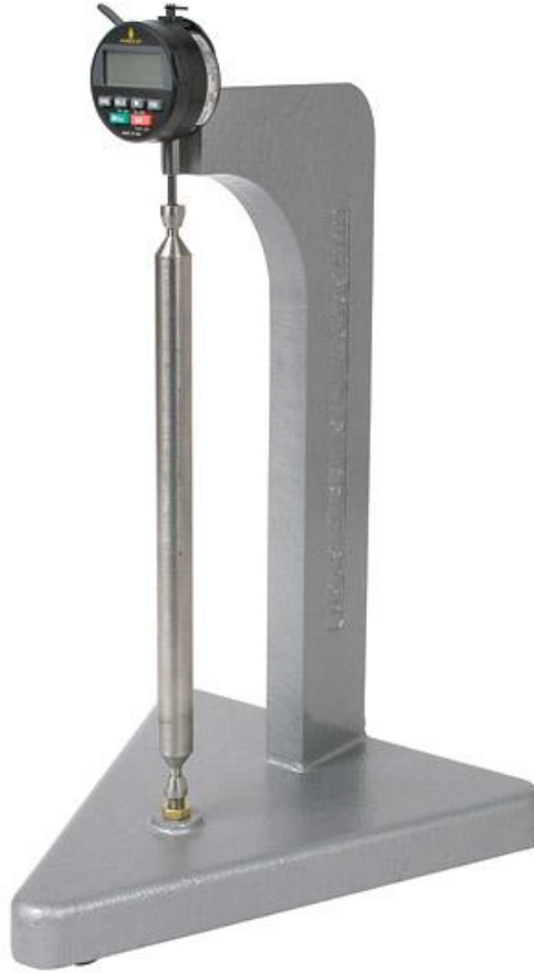
Figure 3.4 Length Comparator with Digital Indicator ( www.humboldtmg.com )
